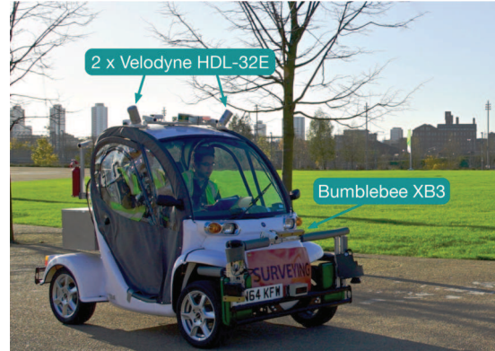
Fig. 8. Mobile research platform: a modified GEM golf cart.
